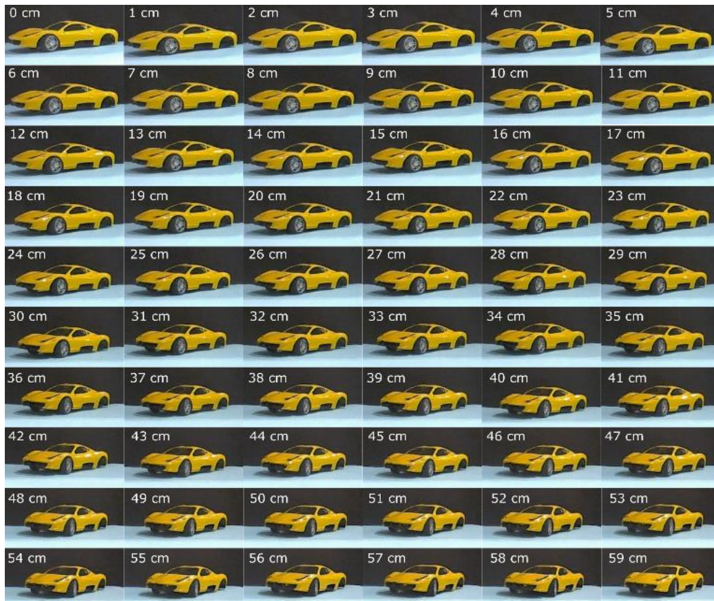
Figure 6: The set of multi-perspective views of a real object i.e. toy car recorded using the developed prototype. 60 views are recorded with camera separation of 1 cm.
